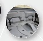
> 3 dedicated dispensing probes: 2 for reagents, 1 for samples-ensuring precision with CV <1% at 0.1 Abs
